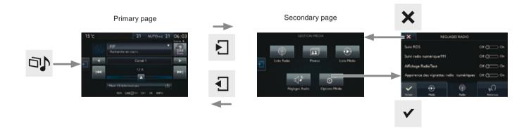
Shortcuts: using virtual buttons in the top band of the touch screen, it is possible to go directly to the choice of audio source, the list of stations (or titles depending on the source) or to the temperature adjustment.
